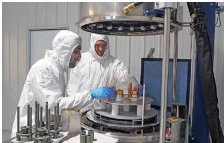
Jerod Day and Bryce Sollazzi prepare subassemblies at the new furnace for VI, Inc.'s first vacuum interrupter design.
